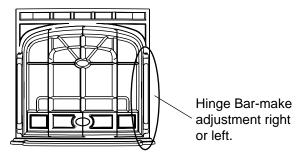
**Figure 8.17** Use a 5/32 in. Allen head wrench and loosen the Allen head bolts. Make necessary adjustment (move hinge to right or left, for proper fit and operation of doors, and retighten Allen bolts.
